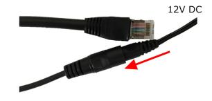
STEP 4: Connect a 12V DC Power Source to the DC POE Injector. You will see two green lights on the DC POE and a light on the AirGateway
