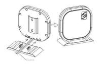
Option 2: Using the built-in bracket, attach the antenna to a flat wall, as show below.
